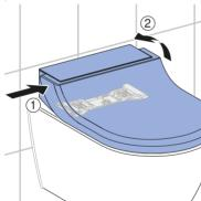
Lift the device as far as the removal limiter permits. Clean the gap between the shower toilet and ceramic sanitary appliance.
