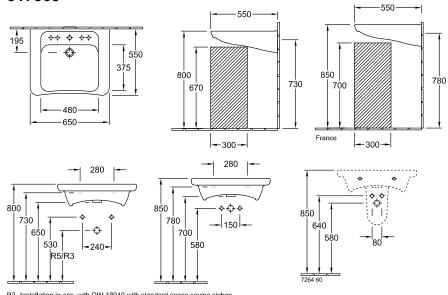
R3 Installation in acc. with DIN 18040 with standard space saving siphon R5 Installation in acc. with DIN 18040 with standard concealed siphon
