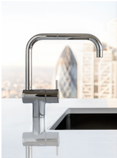
KV1 One-handle mixer with ceramic disc technology, double swivel spout and water saving aerator. Pipe size: 10 mm. Hole cut out size: 32 mm.
